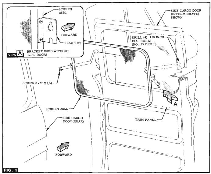
STEP 1 POSITION SCREEN & LOCATE SCREW HOLES BY MEASURING UP FROM TRIM PANEL TO LOWER HOLE OF SCREEN BRACKET. CENTER PUNCH & REMOVE SCREEN. SEE FIG. 1. NOTE Screens must be held tight against door when punching centers.
