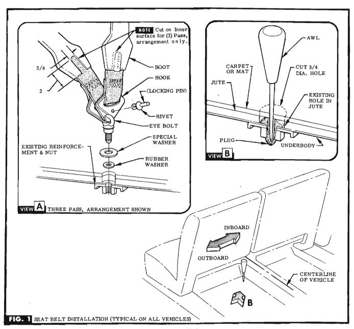
STEP 1 USING DIMENSIONS GIVEN, LOCATE PLUG BY FEELING CARPET OR RUBBER MAT (SLIGHT INDENTATION). PROBE WITH AWL TO LOCATE HOLE IN PLUG. INSERT AWL DOWN INTO PLUG & LEAVE STANDING IN UPRIGHT POSITION, CUT CARPET OR MAT. SEE FIG. 1 & VIEW B.
