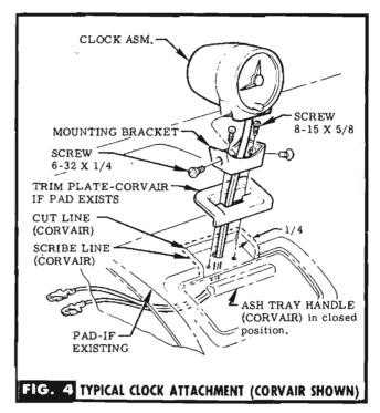
STEP 3 INSERT CLOCK WIRES THRU CENTER HOLE IN MOUNTING BRACKET & TRIM PLATE (IF REQUIRED) & ATTACH BRACKET TO INSTRUMENT PANEL WITH SCREWS. SEE FIG. 4.
