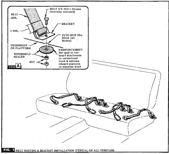
**STEP 1** REMOVE SEAT CUSHION & BACK OR FOLD SEAT FOR ACCESSIBILITY, ALSO TURN BACK FLOOR MAT AT AREA OF INSTALLATION, IF EXISTING. PIERCE & SLIT AREA OF MAT AT BRACKET LOCATIONS.
