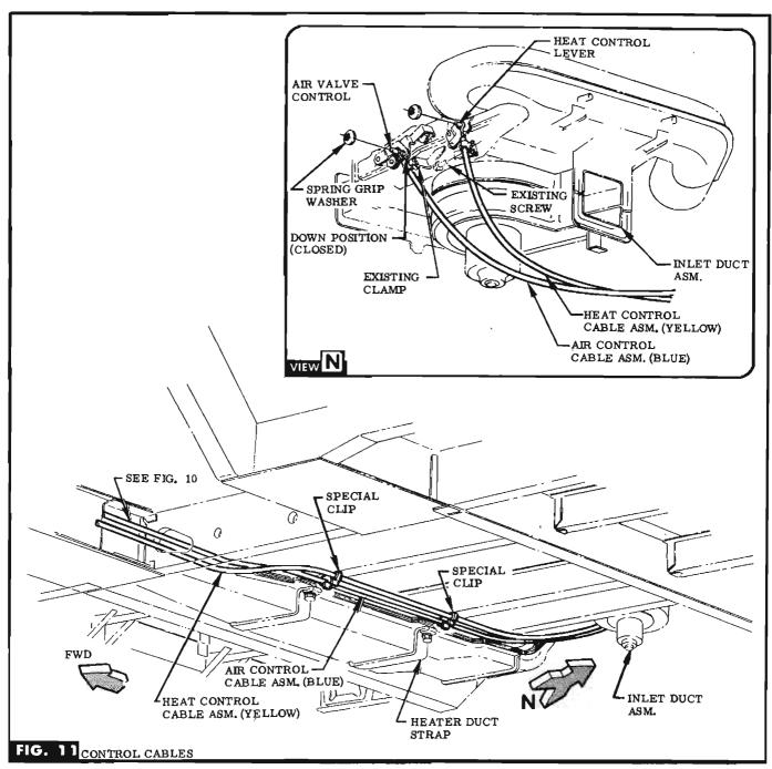
**STEP 57** INSTALL CLIPS (IN BAG B) TO INTERMEDIATE & REAR CROSSMEMBERS ALONG SIDE DUCT STRAP ATTACHMENTS. SEE FIG. 11.
