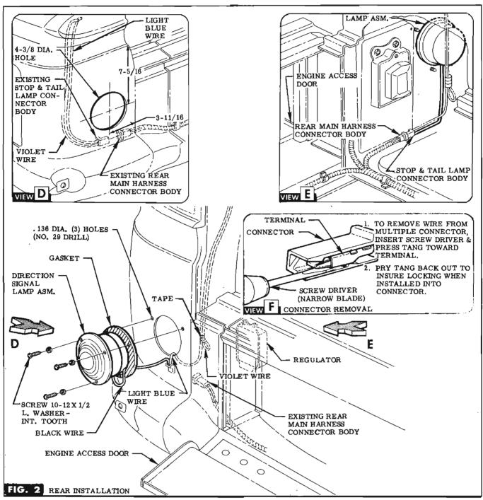
STEP 13 LOCATE, CENTERPUNCH & DRILL HOLE TO DIM-ENSION SHOWN. SEE VIEW D. NOTE If hole saw is used, set saw to 4-1/4 Dia.
