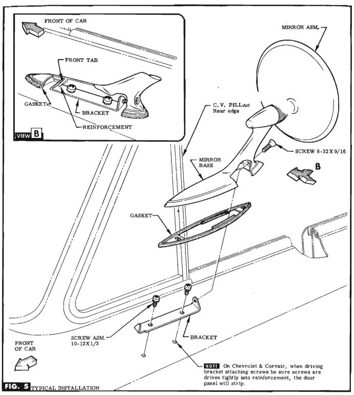
STEP 7 PLACE BRACKET ON DOOR WITH THREADED HOLE IN BRACKET TO REAR. SEE. FIG. 5. NOTE Use (WHITE) bracket on Corvair, (Chevy-except sport coupe & convertible), Truck & Corvair 95. Use (GOLD) bracket on Chevrolet, & (Chevy-sport coupe & convertible).
