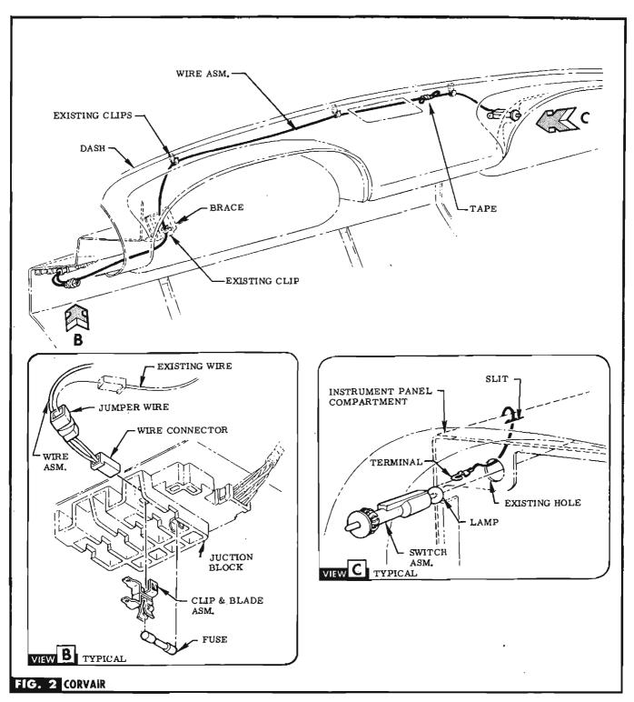
STEP 1a ROUTE WIRE TERMINAL THRU SLIT IN UPPER LEFT HAND CORNER OF INSTRUMENT PANEL COMPARTMENT & THRU HOLE IN UPPER LEFT SIDE OF COMPARTMENT OPENING. SEE FIG. 2 & VIEW C.
