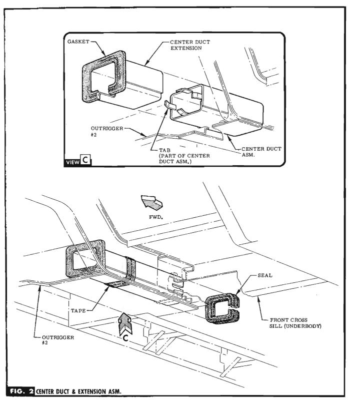
STEP 9 INSTALL GASKET ONTO CENTER DUCT EXTENSION. SEE VIEW  $\mathbf{C}_{\bullet}$
