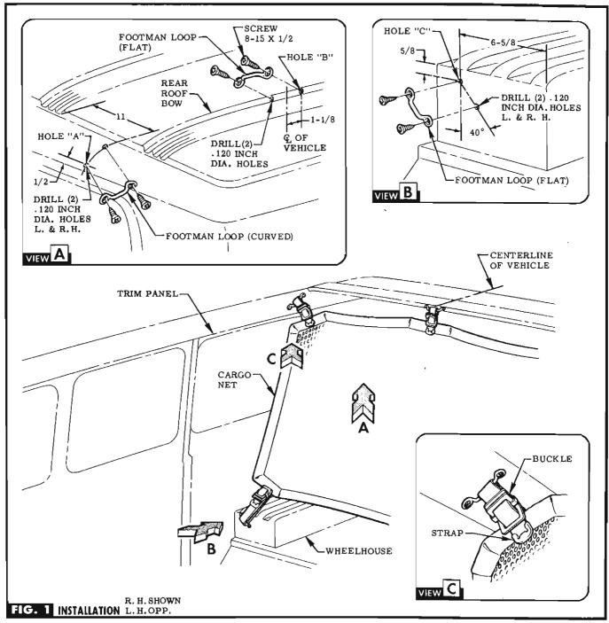
**STEP 1** USING DIMENSIONS SHOWN LOCATE, CENTER PUNCH & DRILL HOLES "A", "B" & "C". FASTEN FOOTMAN LOOPS WITH SCREWS LOOSELY INSTALLED. SEE FIG. 1 & VIEWS A & B.
