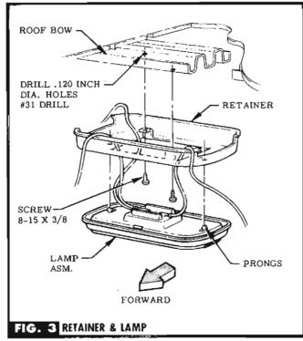
\$1EP 7 POSITION RETAINER ON CENTER OF REAR ROOF BOW & USE IT AS A TEMPLATE TO DRILL HOLES. SEE FIG. 3. CAUTION Do not drill thru roof panel.
