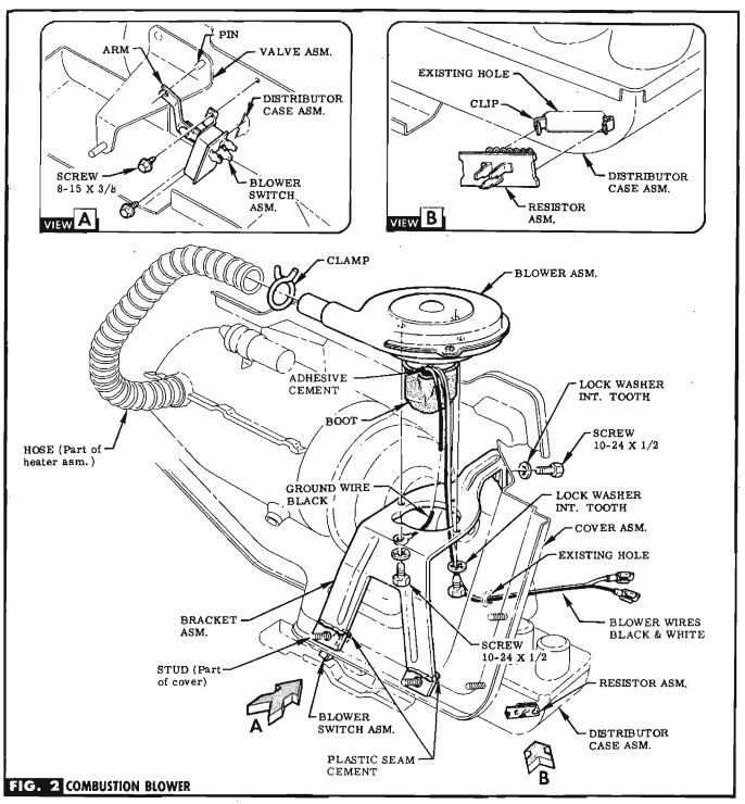
**STEP 6** PLACE BLOWER SWITCH ARM ON VALVE PIN & ATTACH TO DISTRIBUTOR CASE WITH ATTACHING SCREWS PROVIDED (IN BÁG A). SEE VIEW A.
