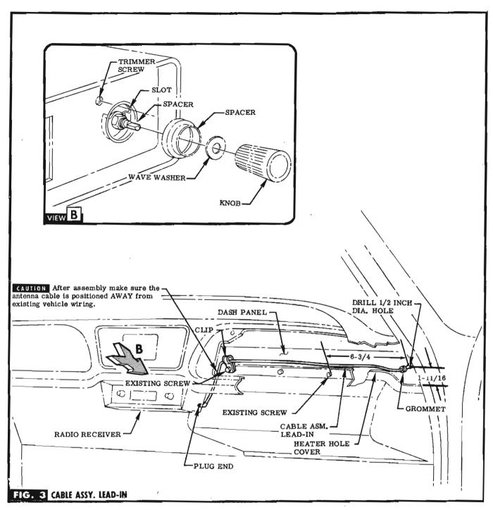
**STEP 8** REMOVE INSTRUMENT PANEL COMPARTMENT. LOCATE & DRILL HOLE IN DASH PANEL FROM INNER SIDE THRU INSTRUMENT PANEL COMPARTMENT OPENING. SEE FIG. 3.
