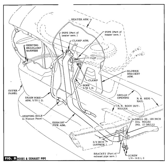
STEP 36 INSERT EXHAUST PIPE THRU EXISTING OPENING IN PLENUM PANEL, FIT CLAMP ASM. PROVIDED OVER TOP & SLIDE EXHAUST PIPE OVER HEATER PIPE. SEE FIG. 8.
