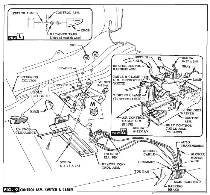
STEP 46 ATTACH SWITCH TO HEATER CONTROL WITH SCREWS (IN BAG A). SEE VIEW M.
