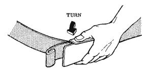
TO LOOSEN BELT TURN BUCKLE OUTWARD
