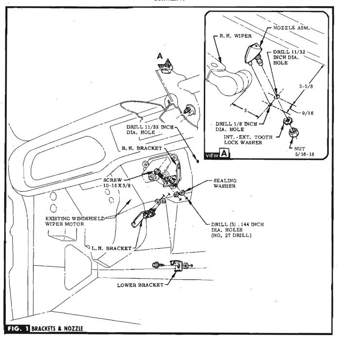
STEP 1 LOCATE EXISTING DIMPLES IN DASH PANEL & DRILL HOLES FOR UPPER R. H. & L. H. & LOWER BRACKETS & GROMMET. SEE FIG. 1. HOIL If heater exists, use lower hole of heater control cables clip for attaching lower bracket.
