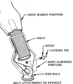
(WITH RIVET IN REMOVED POSITION)
