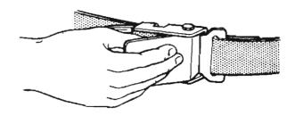
TO LOOSEN BELT TURN BUCKLE OUTWARD
