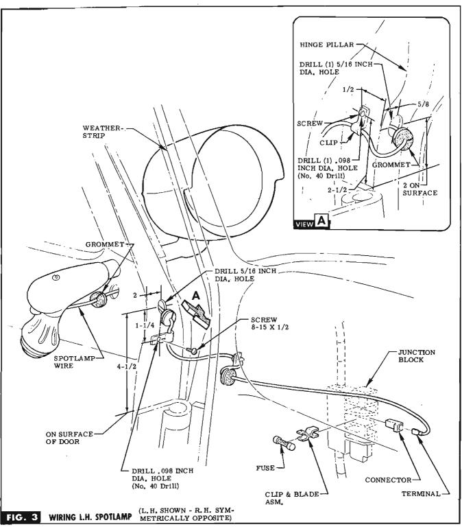
STEP 9 LOCATE, CENTER PUNCH & DRILL HOLES ON FORWARD EDGE OF DOOR & FRONT BODY HINGE PILLAR. SEE FIG. 3 & VIEW A.
