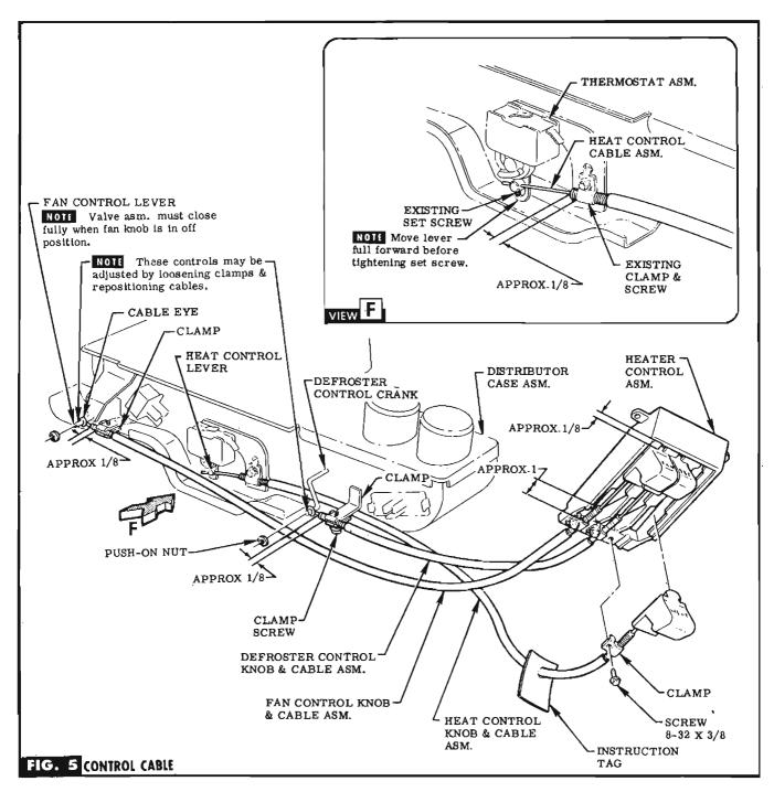
STEP 23 INSERT FAN, DEFROSTER & HEAT CONTROL KNOB & CABLE ASSEMBLIES INTO SLOTS OF HEATER CONTROL. SLIDE CABLE SHEATHS UP INTO SLOTS & SECURE TO DIMENSION SHOWN WITH CLAMPS & SCREWS (IN BAG A). SEE FIG. 5.
