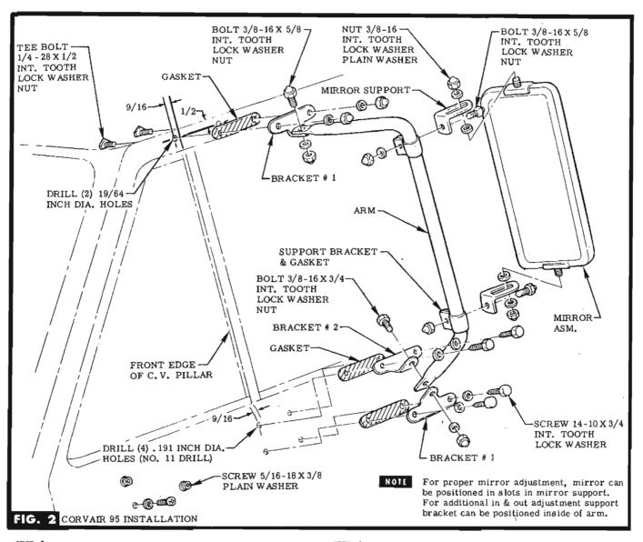
STEP 1a ON L. H. SIDE ONLY, REMOVE & DISCARD EXISTING MIRROR & ATTACHING PARTS, PLUG HOLES WITH PARTS PROVIDED, SEE FIG. 2.
