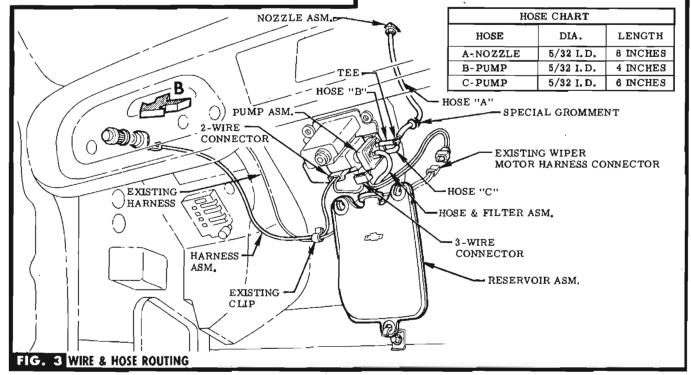
STEP 6 PLACE WIPER MOTOR IN PARK POSITION, RE-MOVE PLASTIC COVER FROM DRIVE SHAFT OF WIPER MOTOR & POSITION CAM ON SHAFT, DISCONNECT MOTOR HARNESS CONNECTOR, SECURE PUMP ASM. TO WIPER MOTOR ASM. WITH SCREWS PROVIDED. SEE FIG. 2. CAUTION Cam follower on Pump must ride on outer surface of Cam & may require that Cam be rotated slightly to allow proper alignment.
