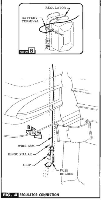
assist routing thru holes & around corners.
