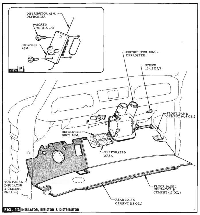
STEP 63 REMOVE EXISTING FLOOR MAT & CEMENT PROVIDED PADS TO UNDERBODY OF FLOOR MAT. CUT OUT PERFORATED AREA. SEE FIG. 1.
